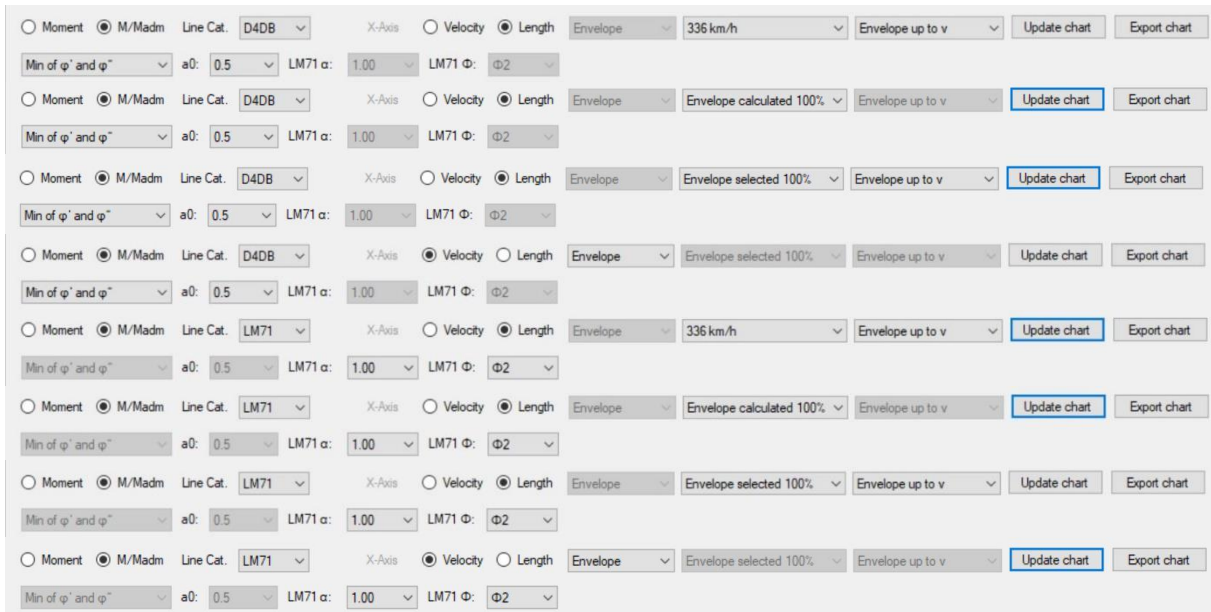
Figure 41: 2-D presentation: Examples of suggested menu settings for M/Madm with line category D4DB as reference and view options for “intersection”, “envelope up to v” and “envelope 100%”
